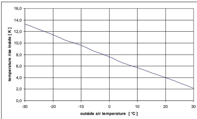
Inside - outside – difference temperature by using the heating.
