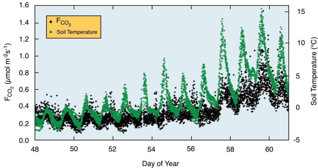
An example of time series data for soil  $\text{CO}_2$  flux ( $F_{\text{CO}_2}$ ) obtained with a 16-chamber system at Lincoln, Nebraska. Soil temperature data at a depth of 5 cm from each chamber are also shown. For more information on data collected from a multiplexed system, visit [www.licor.com/multiplex](http://www.licor.com/multiplex).
