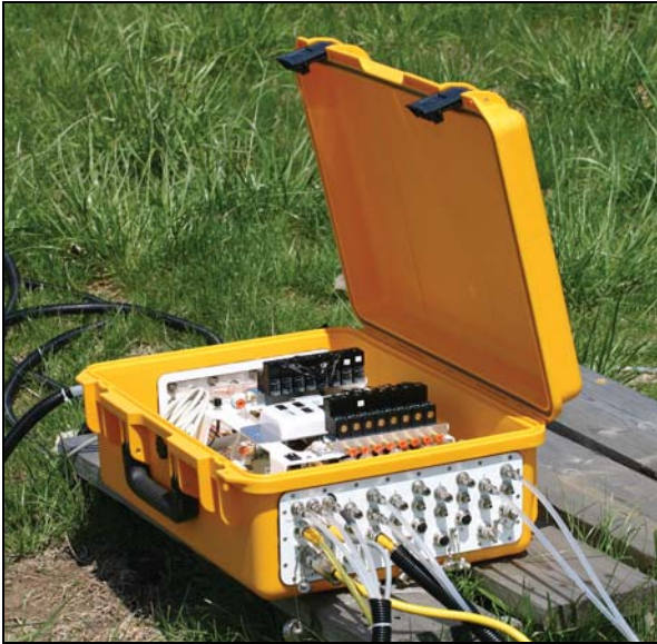
Figure 10-8. Cable connections for LI-8150 and a soil chamber.
