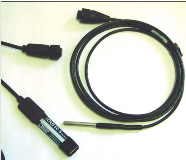
Figure 7-4. The 8100-104/C use dedicated soil moisture (left) and soil temperature (right) probes which have 8-pin connectors for direct attachment to the chamber. These probes are active only when the 8100-104/C is used in conjunction with the LI-8150 Multiplexer.
