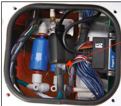
Figure 2-4. To remove the Ethernet adapter card, eject the card, and disconnect the cable at the junction shown.
