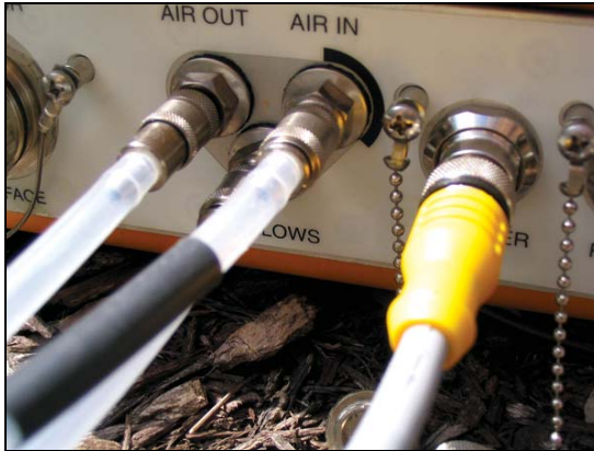
Figure 6-5. Survey Chamber hose connections.
