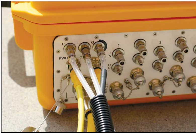
Figure 10-7. Attach the air hoses and control cable.
