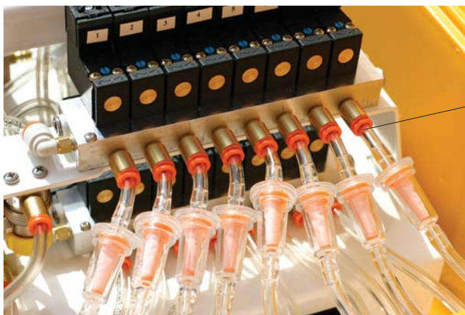
Figure 10-20. Note orientation of filters. Attach nearest the solenoids first, and cut the tubing at the other end to length.
