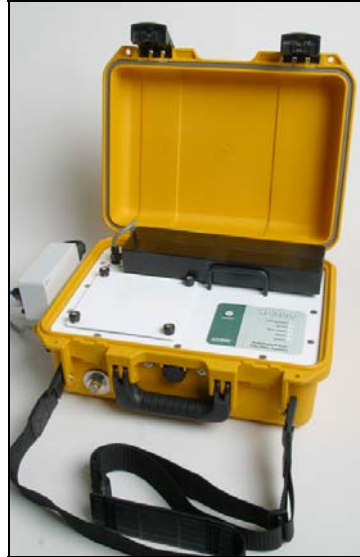
Figure 1-1. Analyzer Control Unit, with 6400-03 Rechargeable Battery, Auxiliary Sensor Interface, and shoulder strap.
