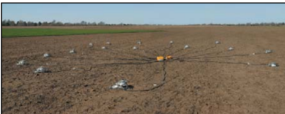
Figure 10-1. As many as 16 chambers can be connected at one time, with a measurement diameter of up to 30 m.
