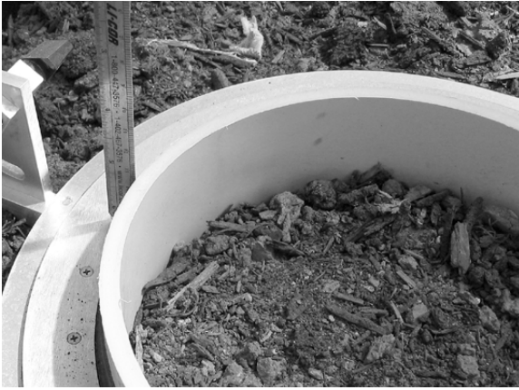
Figure 2-18. Chamber offset measurement using Survey and Long-Term Chambers.
