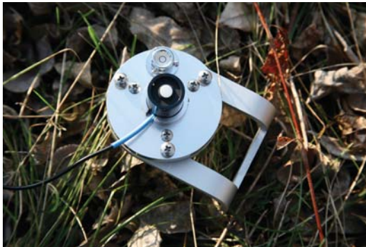
Figure 4-5. The 8100-604 Leveling Stake (left) is used to mount and level the LI-190 Quantum Sensor for measuring PAR near the 8100-104C Clear Chamber. In multiplex mode, the LI-190 requires the 392-08577 plug with bare wire leads (right) between the amplifier and the chamber.
