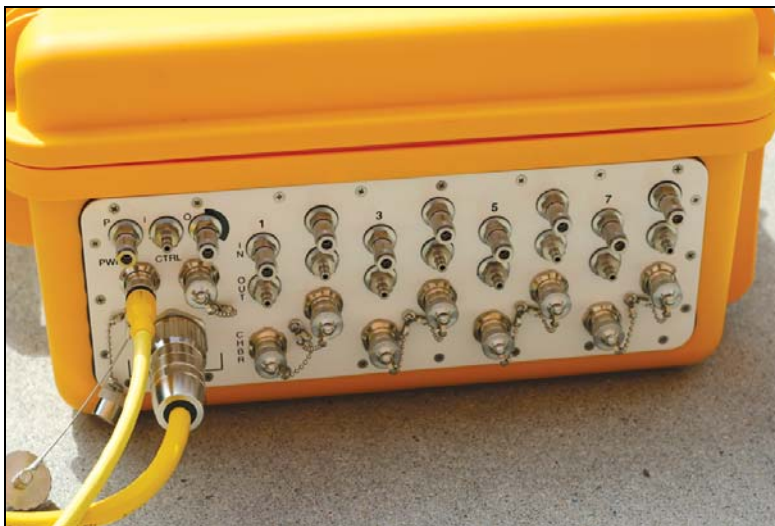
Figure 10-6. Attach the bulkhead connector and power cable.
