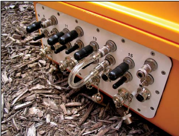
Figure 10-10. In the absence of extension tubing, the leak test fixture is attached between the air inlet and outlet ports (port #14 shown).
