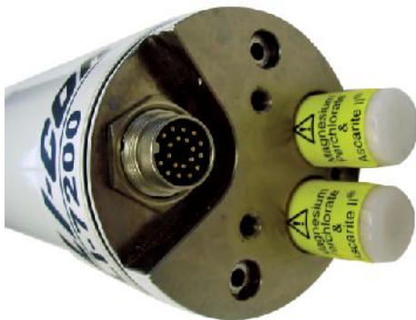
Figure 5-4. Insert the recharged bottles cap first. Make sure the caps have holes in the top.
