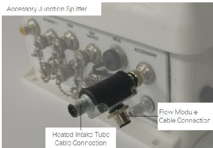
Figure 2-3. The Accessory Junction Splitter is used for all heated intake tubes.
