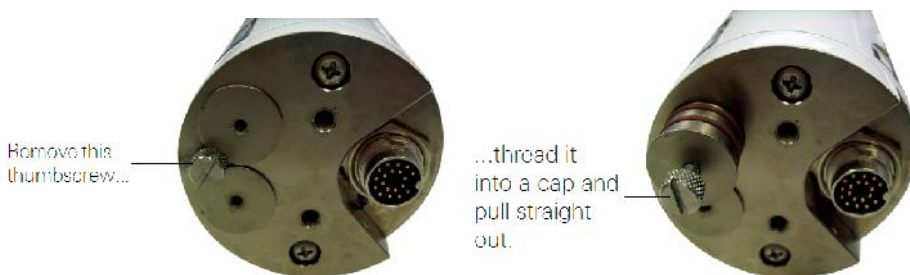
Figure 5-3. Remove the thumbscrew, thread it into the bottle covers, and then pull straight
