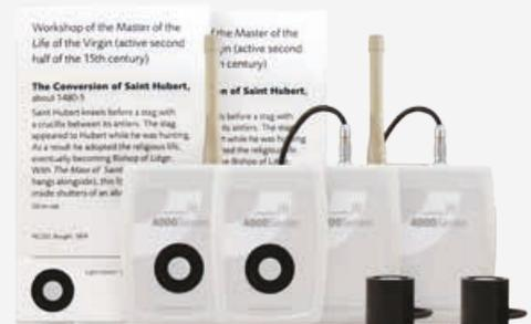
The ML4000 Lux/UV range (data loggers and radio transmitters options available) monitor light to assist in preserving sensitive materials such as print, drawings, fabrics, oil paintings and wooden objects.
