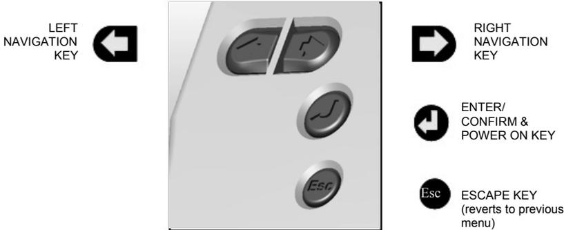
To use the 2020/2040 control panel press
