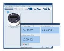
In the Logger control window click at **Meter-mode**, if you wish to see actual readings of the datalogger.
