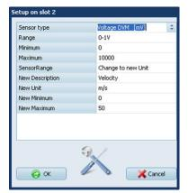
InfraLog automatically defines a **minimum** and a **maximum** of the electrical sensor range. You may alter this, if needed.
