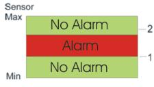
There is one alarm range for the selected channel. If the sensor value is higher than the (Alarmthreshold1 ± Hysteresis) and lower than (Alarmthreshold2 ± Hysteresis) the logger goes into alarm.
