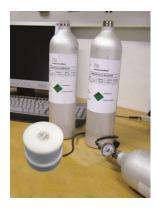
Driesen+Kern GmbH offers a zero-gas as well as a regulator and a calibration adapter as a calibration kit.
