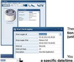
These settings are Logger Start condition, logger stop condition, interval (unit/value) and a run description.
