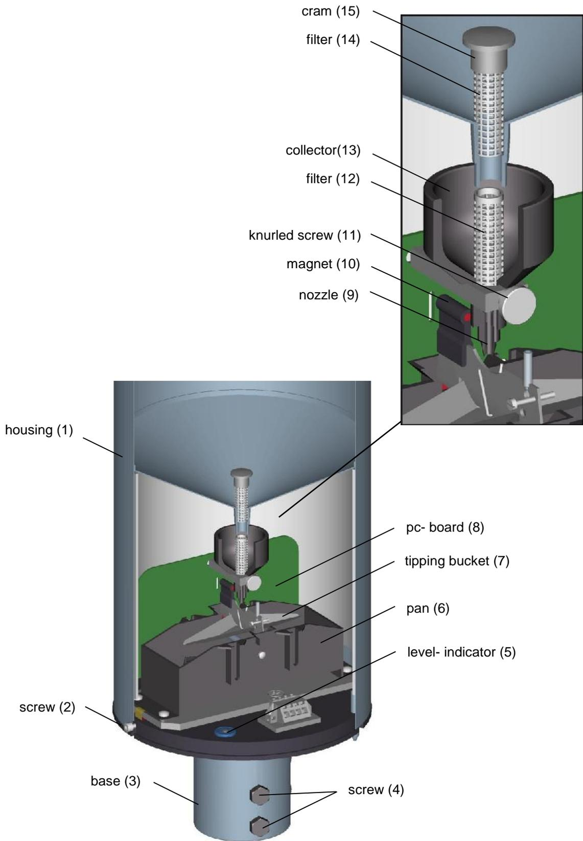
**Figure 1: Instrument construction**
