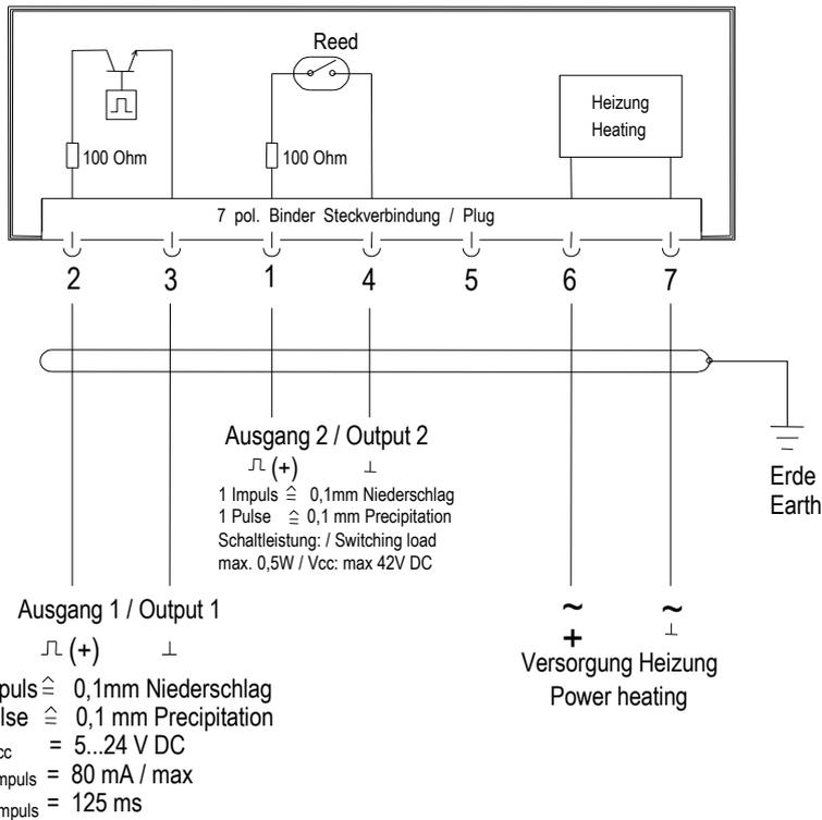
View on the soldered joint of the counter plug.
