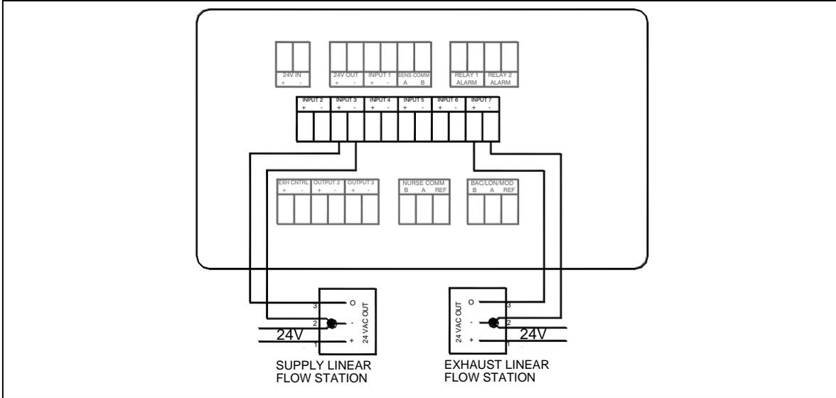
Figure 25. Optional Supply & Exhaust Linear Flow Station Wiring to Model RPC30
