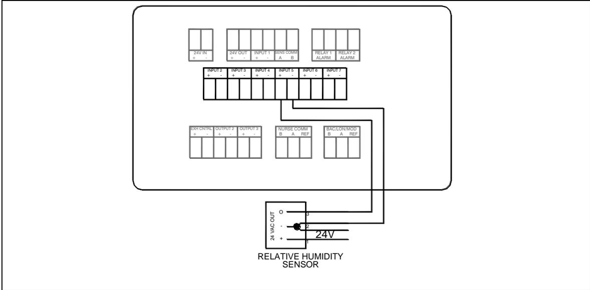
Figure 32. Optional Relative Humidity Sensor Wiring to Model RPC30
