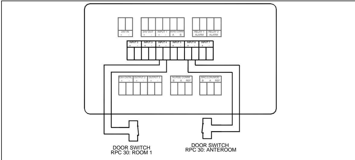
**Figure 27. Optional Door Switch Wiring to Model RPC30**
