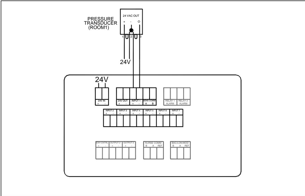
Figure 21. Wiring Diagram – Pressure Transducer Sensor to Model RPC30
