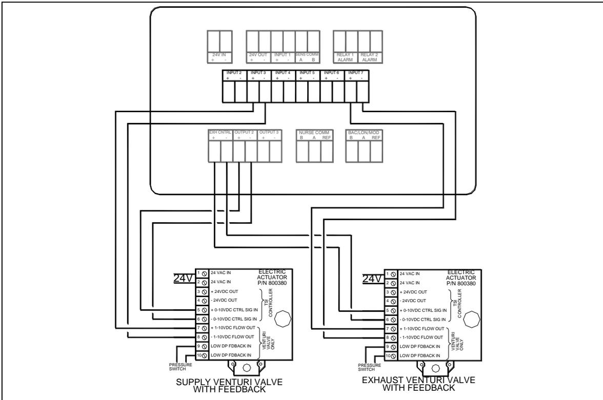
Figure 26. Optional Supply & Exhaust Venturi Valve Wiring to Model RPC30
