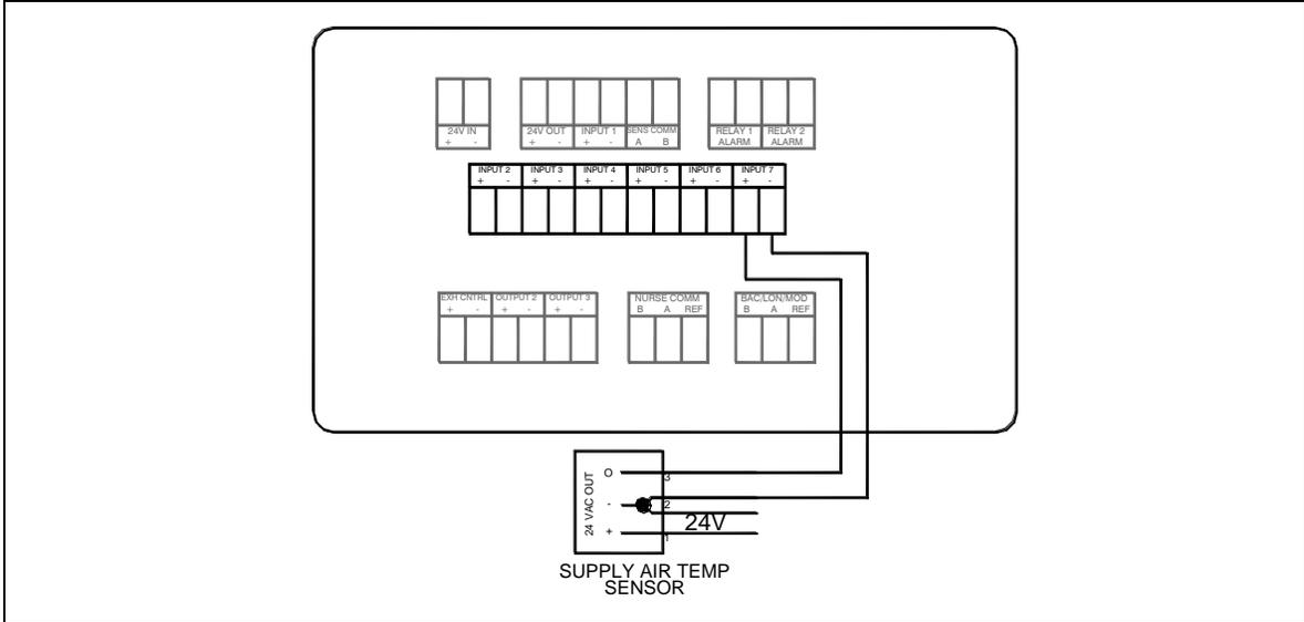
Figure 34. Optional Supply Air Temperature Sensor Wiring to Model RPC30
