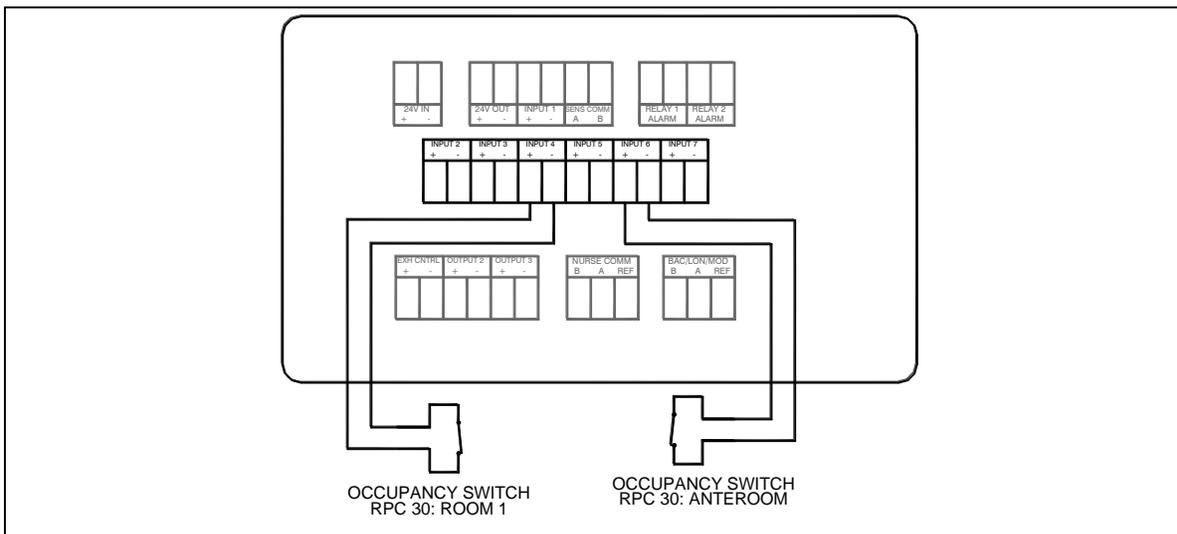
**Figure 28. Optional Occupancy Sensor Wiring to Model RPC30**
