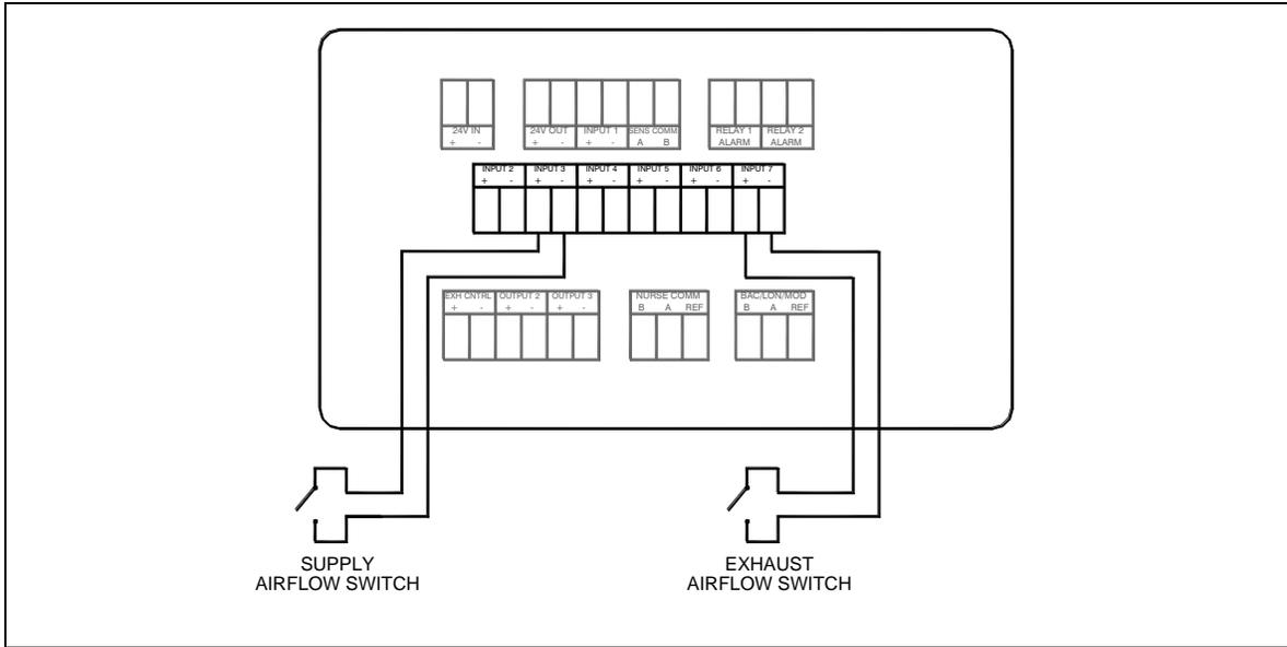
**Figure 23. Optional Supply & Exhaust Flow Switch Wiring to Model RPC30**
