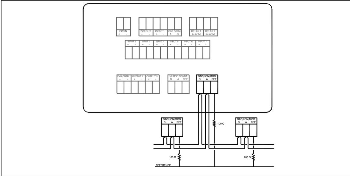
**Figure 38. Optional Modbus and BACnet MS/TP Communications Wiring to Model RPC30**
