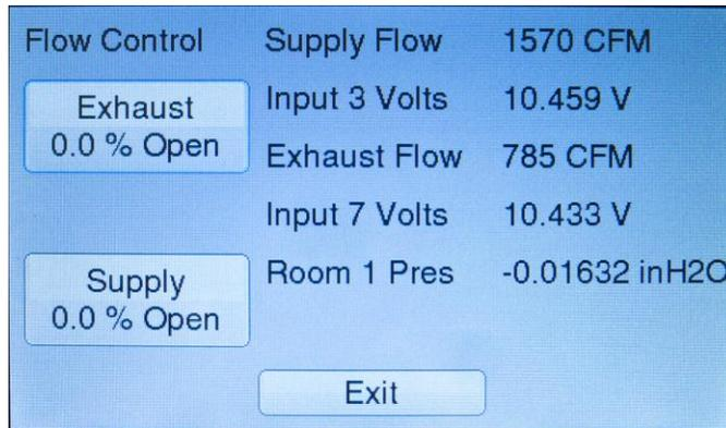
**Figure 13. Flow Control screen in Diagnostics menu**
