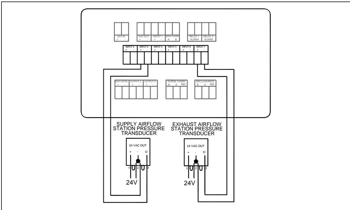
**Figure 24. Optional Supply & Exhaust Pressure-Based Flow Station Wiring to Model RPC30**
