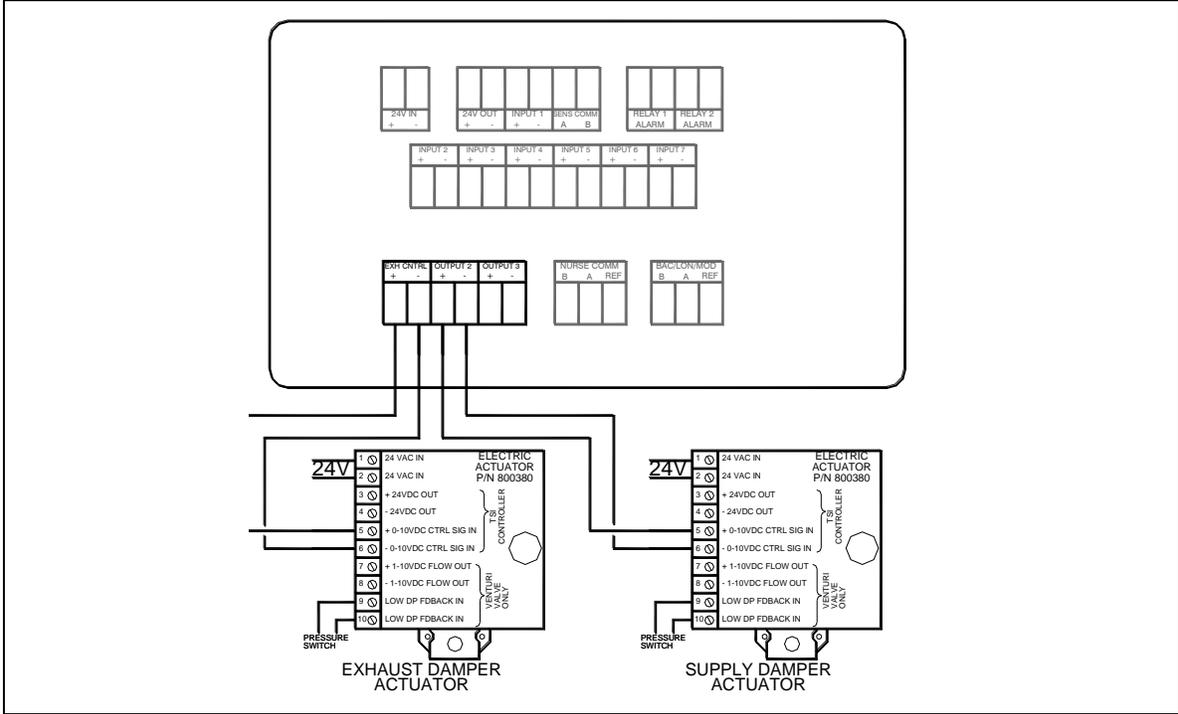
Figure 35. Optional Supply & Exhaust Actuator Wiring to Model RPC30
