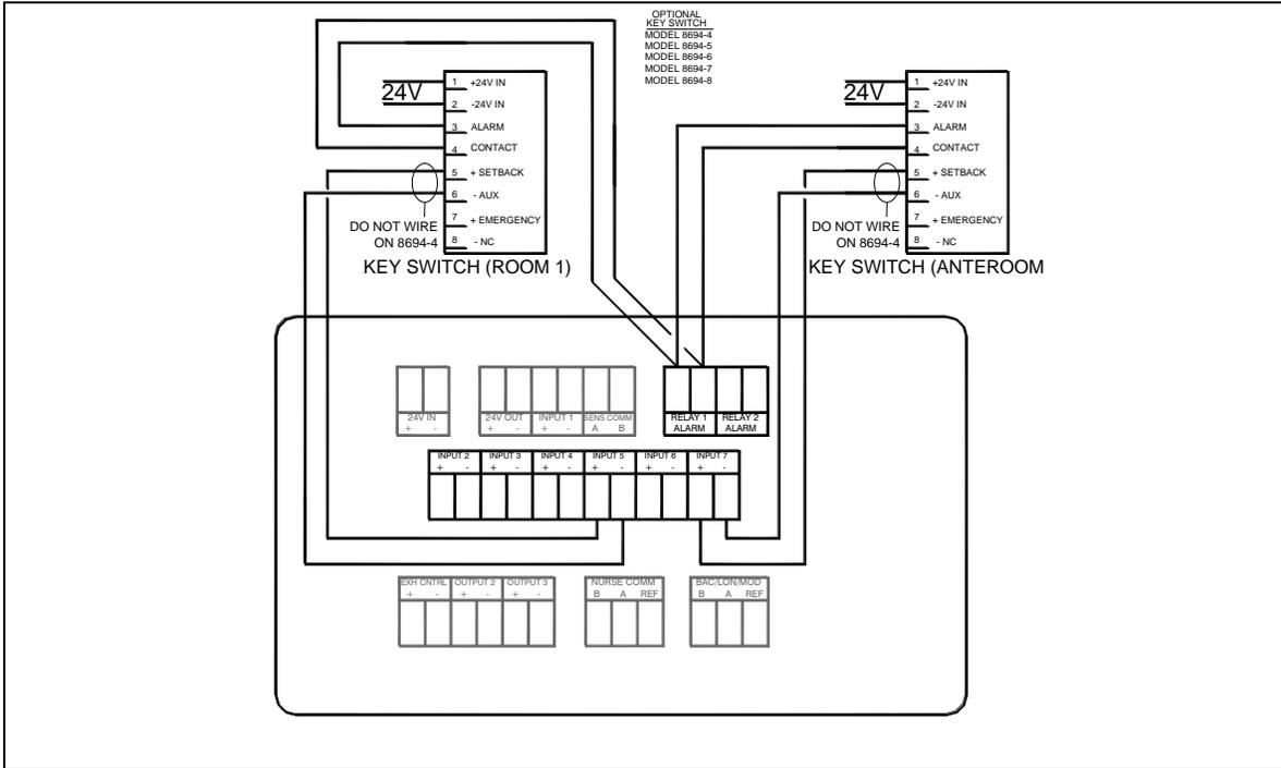
Figure 30. Optional Keyswitch Wiring to Model RPC30
