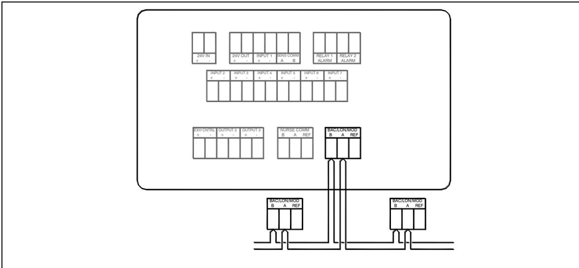
**Figure 39. Optional LONworks Communications Wiring to Model RPC30**
