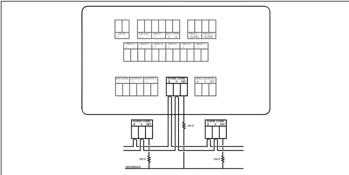
Figure 37. Wiring Diagram – Optional Nurses Station Communications Wiring to Model RPC30
