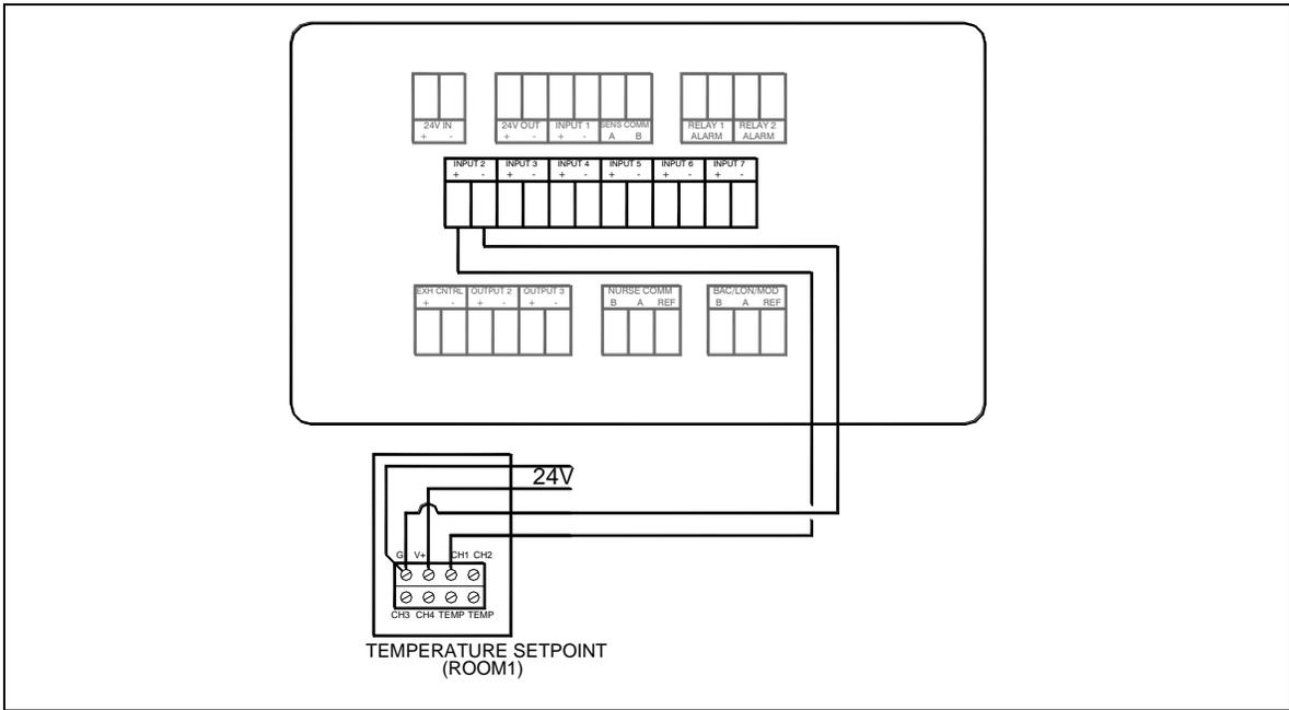
Figure 33. Optional Temperature Setpoint Wiring to Model RPC30
