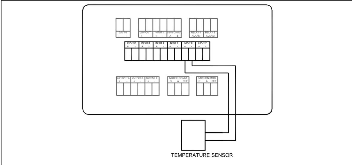
Figure 29. Optional Temperature Sensor Wiring to Model RPC30
