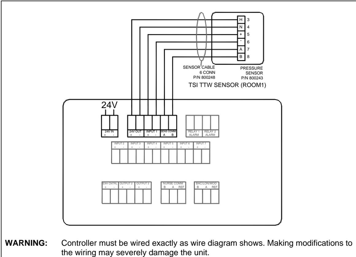
**Figure 19: Wiring Diagram –Through-The-Wall Sensor Wiring to Model RPC30**
