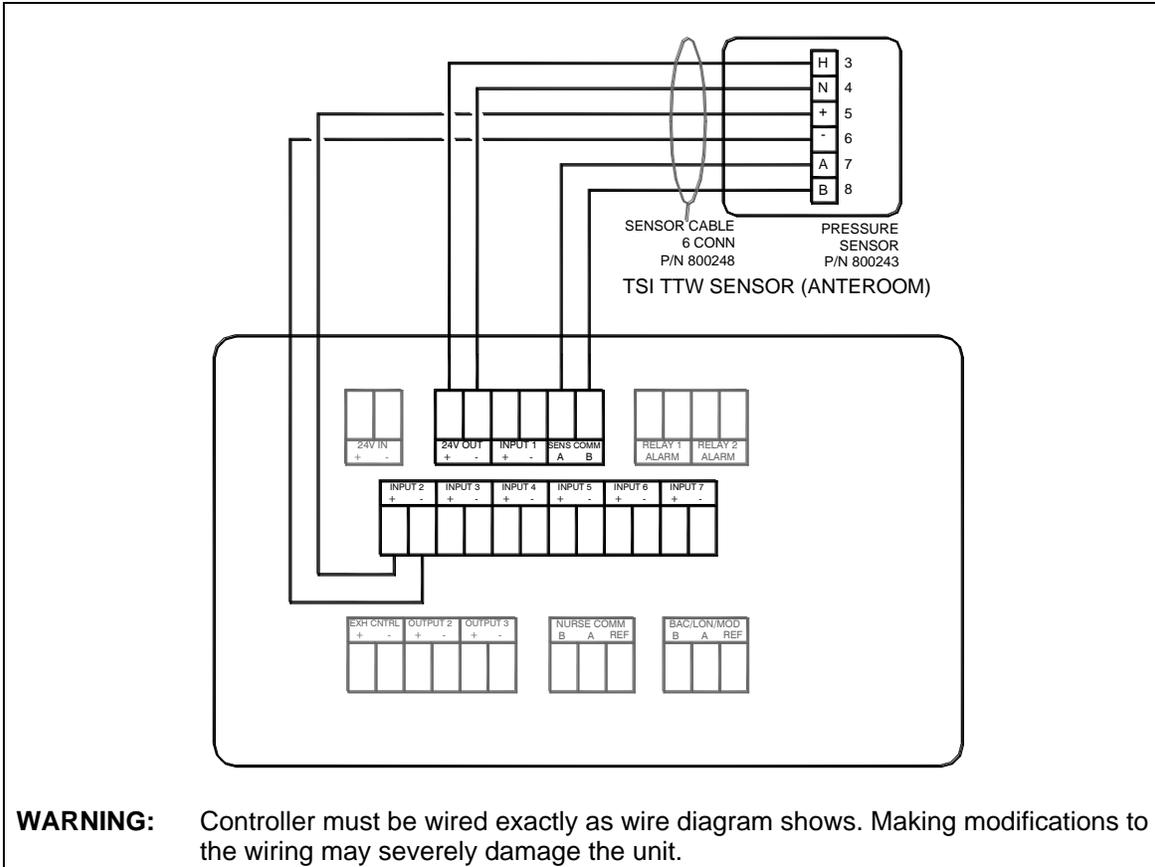
**Figure 20: Optional Anteroom Through-The-Wall Sensor Wiring to Model RPC30**
