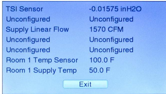
Figure 16. View Inputs screen in Diagnostics menu
