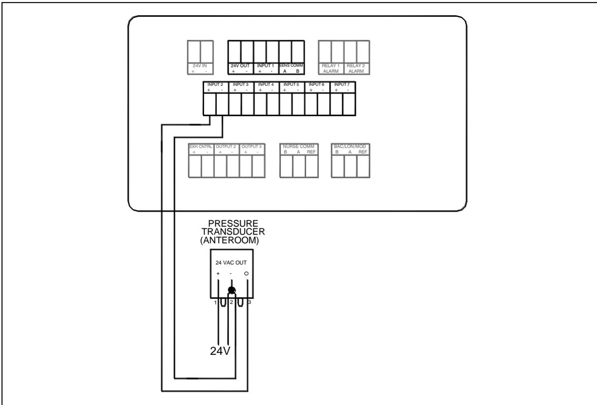
Figure 22. Optional Anteroom Pressure Transducer Sensor Wiring to Model RPC30
