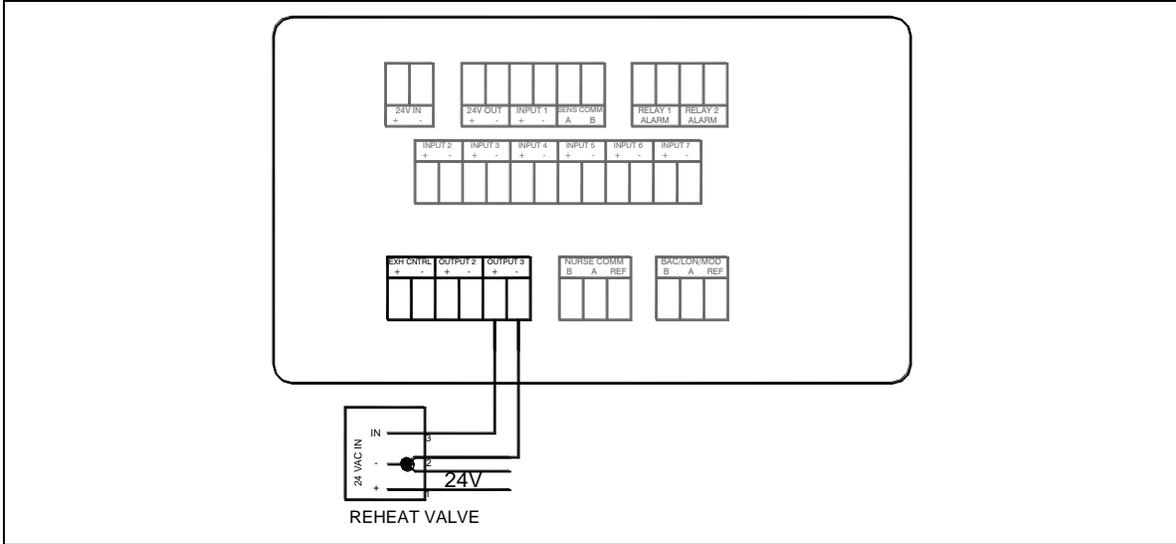
Figure 36. Optional Reheat Actuator Wiring to Model RPC30.
