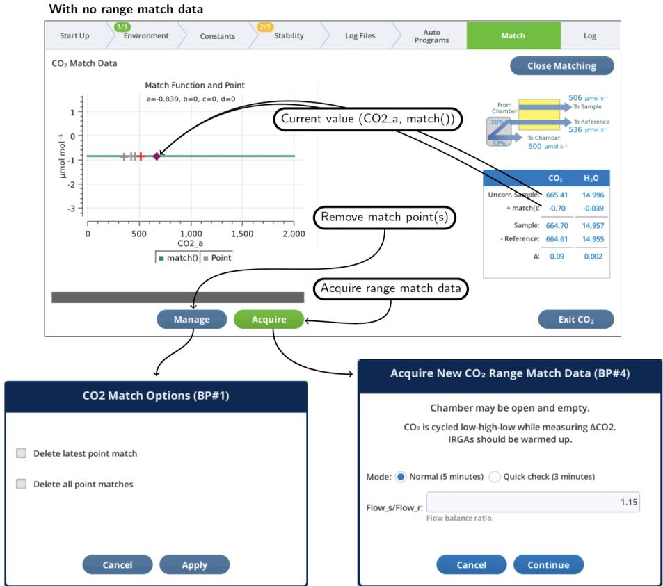
Figure 1-41. The CO<sub>2</sub> Match Data screen shows an expanded version of the CO<sub>2</sub> graph.
