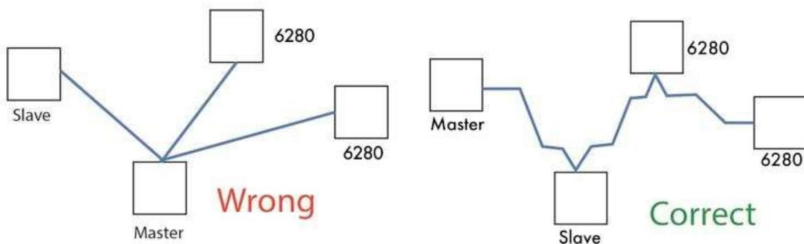
Some there is lack of space in a component, not enough ways in to the terminals, or the installation is smother having a multi-cable out from the component to a junction box. The problem with that is that single cable going between the junction box and the unit can act as a antenna and increase the risk of having com problems. If you must install with junction boxes, make the one cable going in to the unit as short as possible, use twisted pair for the modbus wires.
