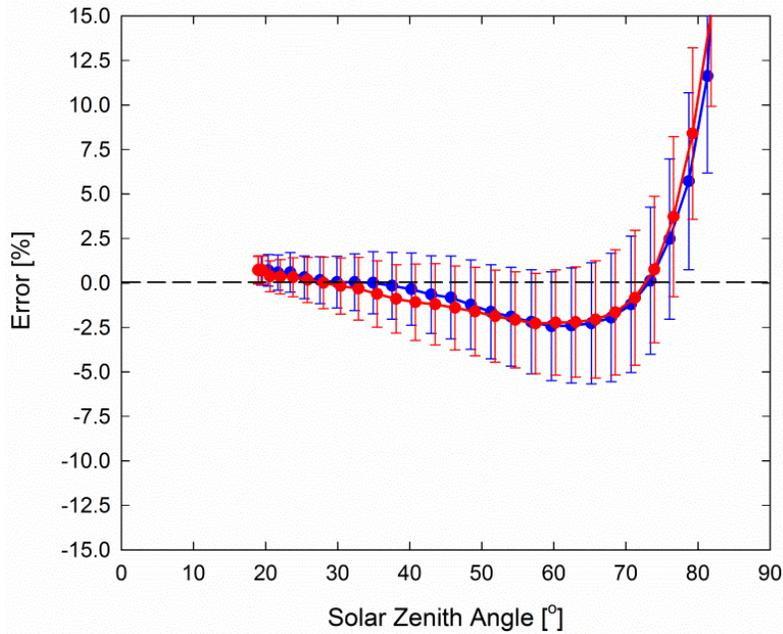
Mean cosine response of twenty-three SQ series quantum sensors (*error bars represent two standard deviations above and below mean*). Cosine response measurements were made by direct side-by-side comparison to the mean of four reference thermopile pyranometers, with solar zenith angle-dependent factors applied to convert total shortwave radiation to PPFD. Blue points represent the AM response and red points represent the PM response.
