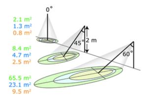
A simple FOV calculator for determining target dimensions based on infrared radiometer model, mounting height, and mounting angle, is available on the Apogee website: <a href="http://www.apogeeinstruments.com/using-your-apogee-instruments-infrared-radiometer/">http://www.apogeeinstruments.com/using-your-apogee-instruments-infrared-radiometer/</a>.
