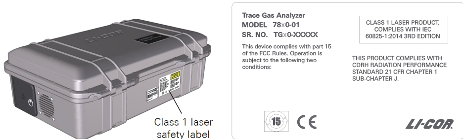
Figure B-1. The Class 1 laser safety label is affixed to the back of the case.
