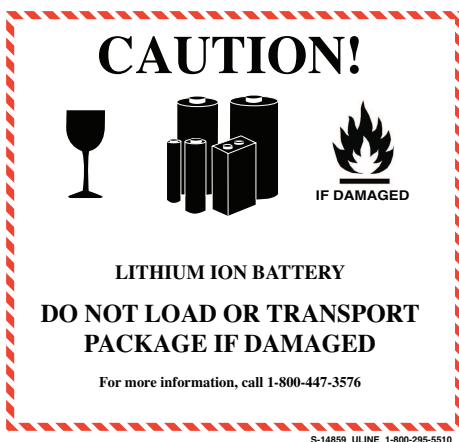
Figure 2-4. Example of Lithium Ion battery handling label. You can download a full-size copy from https://licor.box.com/v/Li-Ion-Shipping-Label .
