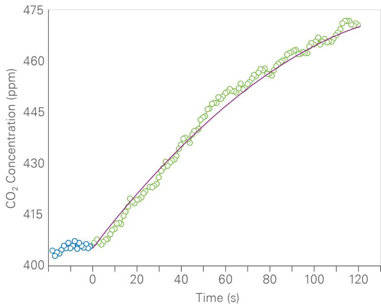
Figure 1. The CO<sub>2</sub> concentration in the chamber begins to increase the moment the chamber closes. As a result, the flux begins to decrease, indicated by the slope ( $\partial C'/\partial t$ ) that decreases with time. Blue circles represent the pre-measurement CO<sub>2</sub> concentration; green circles represent the concentration during the measurement.
