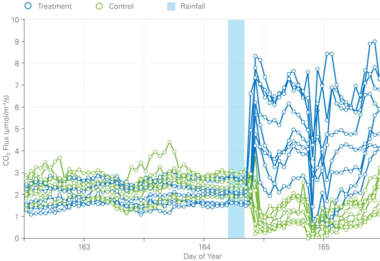
Figure 5. Soil CO<sub>2</sub> flux measurements collected with a 16-chamber system over a cornfield. Treatment plots had crop residue on the soil surface and control plots had no residue. The vertical blue bar represents a 29-mm rain event. Data indicate that for this particular research site, the response of soil CO<sub>2</sub> flux to a rainfall event depends on whether there is crop residue at the soil surface or not.
