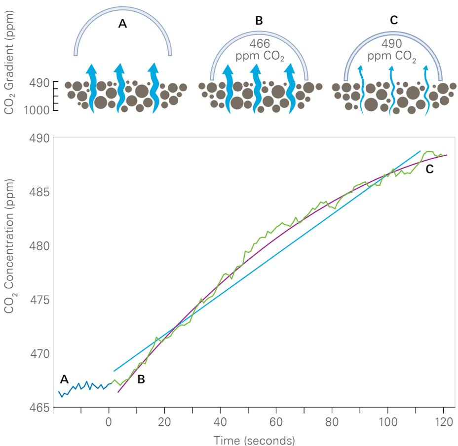
Figure 4. The baseline concentration (A), beginning of the measurement (B), and end of a measurement (C). The LI-8100A and SoilFluxPro™ Software compute the flux from the slope at point B. The red line is the exponential fit, while the blue line is the linear fit.
