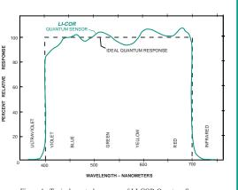
Figure 1. Typical spectral response of LI-COR Quantum Sensors vs. Wavelength and the Ideal Quantum Response (equal response to all photons in the 400-700 nm waveband).
