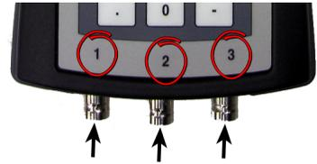
Figure 1-4. Light sensor input ports
