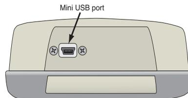
Figure 1-3. Mini-USB port for data transfer and for optional AC power.
