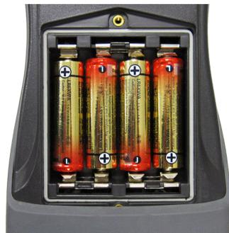
Figure 1-1. "AA" batteries installed.
