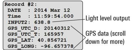
Figure 4-3. Logged data screen for a single record.
