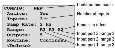
Figure 3-4. Configuration screen with Standard Modes sampling rate greater than 3 Hz total (2 Hz x 3 input ports = 6 Hz total). The "Range:" line displays ranges for input ports 1, 2, and 3 from left to right.
