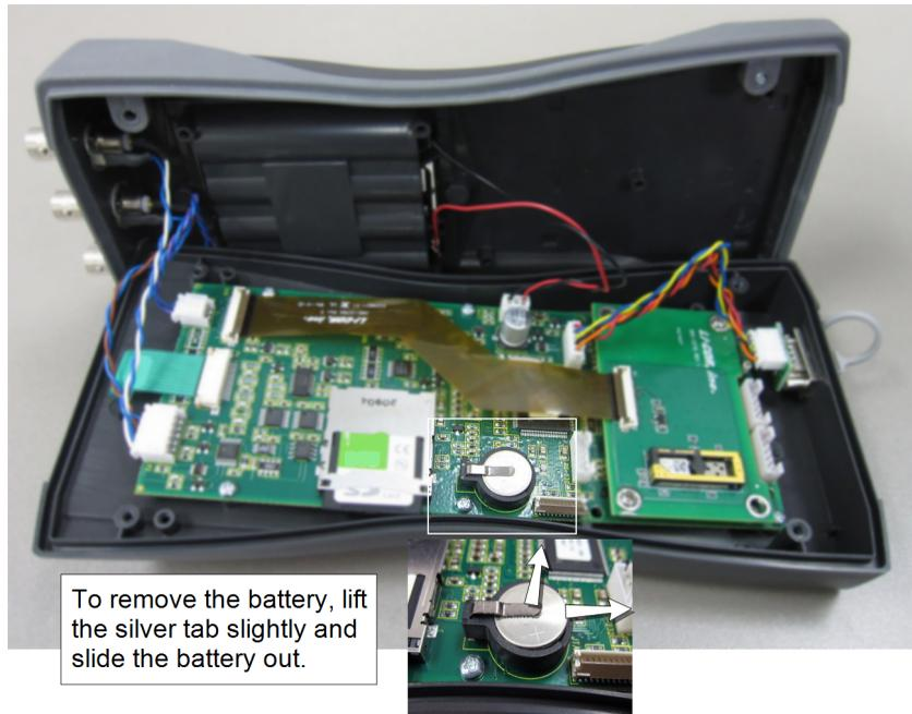
Figure C-1. Replacing the Internal lithium backup battery.
