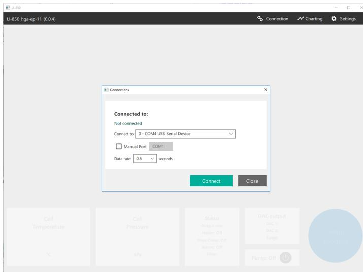
Click the **Connection** button in the upper right of the display. Select your instrument from the list, set the data rate, then click **Connect**. Data will populate the window after connecting. You can enter the COM port manually by checking Manual Port and setting the port number (COM#).
