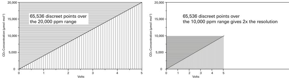
Figure 2-1. The resolution of the analog outputs depends upon the range. If the DACs are configured to output data over the full 0 to 20,000 ppm range, the data output over the DACs will have lower resolution (left). If the DACs are configured to output data over a narrower range (for example, 0 to 10,000 ppm as shown on the right), the data output over the DACs will have higher resolution.
