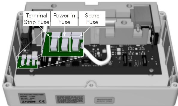
**3** Using a needle-nose pliers, grasp the blown fuse and remove it from the holder.
