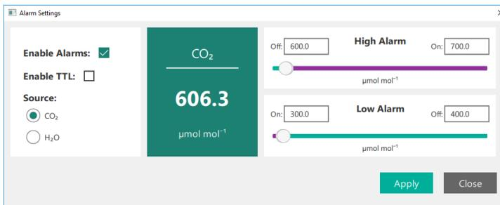
Figure 2-3. The **Alarm Settings** window is where you configure alarms. The settings shown here will give the behavior shown in Figure 2-2 above.
