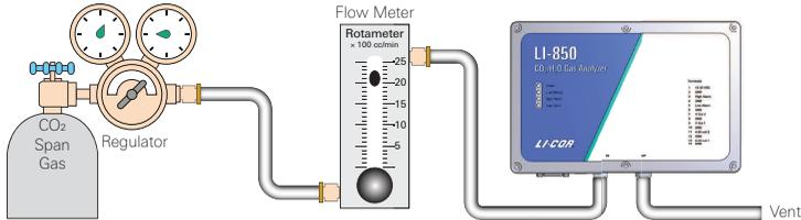
**5** Enter the CO<sub>2</sub> concentration of the span gas into the software
