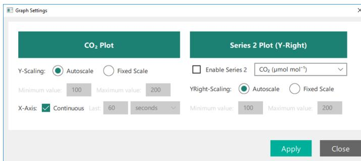
The graphs display a fixed variable: CO<sub>2</sub> and H<sub>2</sub>O with the LI-850. You can configure the settings for each graph and add a second variable. The options are:
