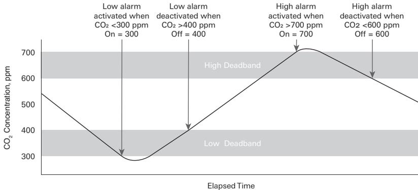
Figure 2-2. An alarm is triggered when a concentration is outside of a threshold. For example, the low alarm is activated if the concentration drops below 300 ppm and is deactivated when the concentration rises above 400 ppm. The high alarm is activated if the CO<sub>2</sub> concentration exceeds 700 ppm. The alarm remains activated until the concentration drops below 600 ppm.
