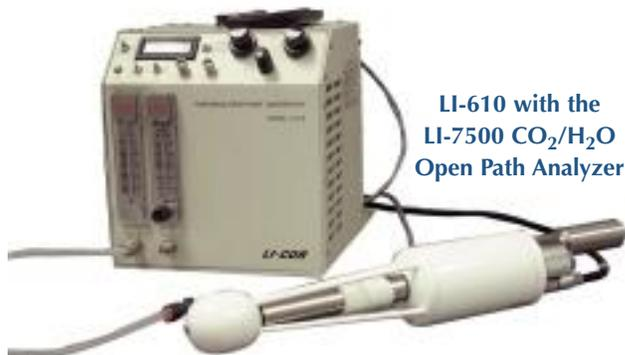
LI-610 with the LI-7500 CO<sub>2</sub>/H<sub>2</sub>O Open Path Analyzer
