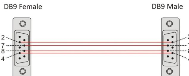
**Figure 112** Building an extension cable
