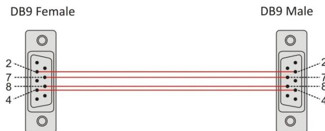
Figure 112 Building an extension cable
