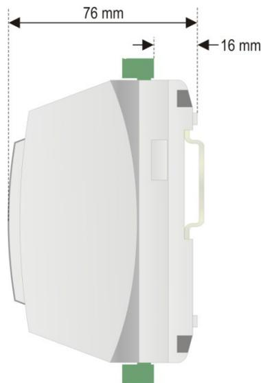
Figure 7 Dimensions of FieldLogger side with HMI module
