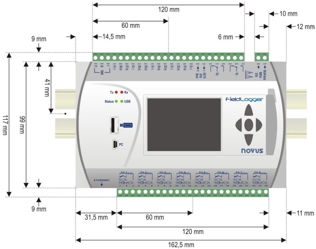
Figure 6 Dimensions of the FieldLogger with HMI module
