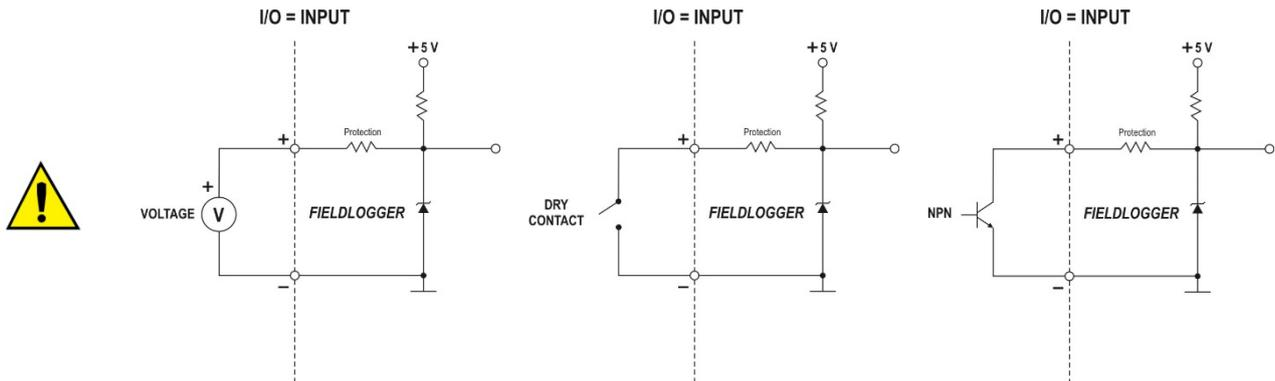
Figure 15 Voltage connection
