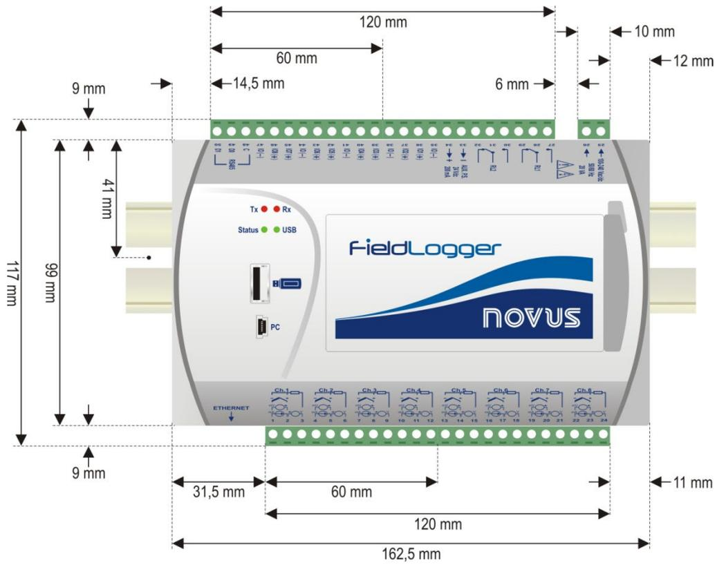
Figure 4 Dimensions of the FieldLogger without HMI module
