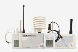
The ML4106, ML4109, ML4114 and RFBug (data loggers and radio transmitter options available) are ideal for humidity measurement to prevent damage to organic materials, such as paintings, sculptures etc.
