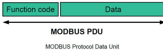
The mapping of MODBUS protocol on a specific bus or network introduces some additional fields on the Protocol Data Unit. The client that initiates a MODBUS transaction builds the MODBUS PDU, and then adds fields in order to build the appropriate communication PDU.
