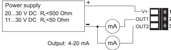
**Important:** The EE210-HT6 (4...20 mA, two-wire) with display operates correctly only if both outputs are connected.
