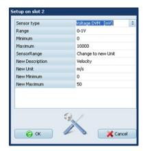
InfraLog automatically defines a **minimum** and a **maximum** of the electrical sensor range. You may alter this, if needed.
