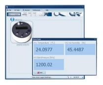
In the Logger control window click at **Metermode**, if you wish to see actual readings of the datalogder.
