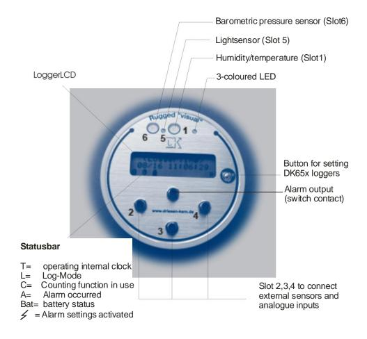
The logger uses sensor slots to which external sensors may be connected to. Some of our sensors are combined sensors (for example humidity and temperature). Such a combined sensor for example RFT-325 Sensors can be connected to a single slot.
