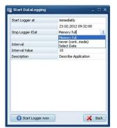
If **Memory full** is selected the logger stops taking new readings when the memory is full.
