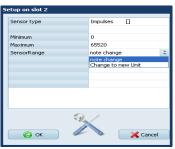
Here you can choose which sensor is connected to slot 2. If you are using one of the standard sensors for the rugged loggers, simply select the corresponding sensor type.
