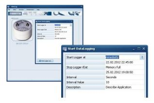
These settings are Logger Start condition, logger stop condition, interval (unit/value) and a run description.
