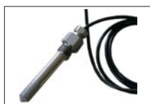
DKRF370-325 Humidity-/temperature sensor for pressure applications max. 100bar, G3/8" thread, Range -20/+80°C L=100mm, D=13mm
