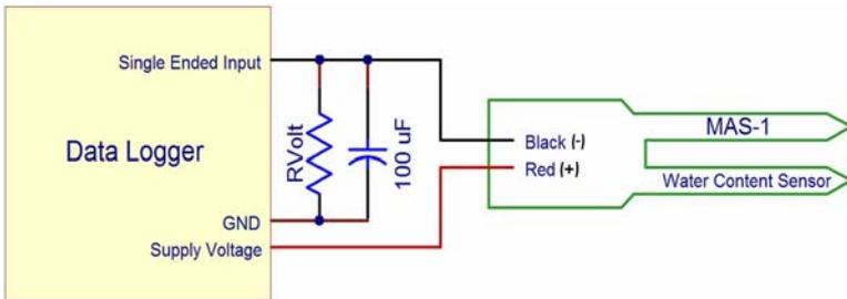
Figure 3 - Wiring connection for devices without current inputs
