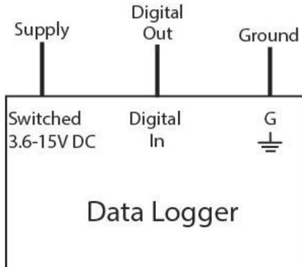
Figure 3: Wiring Diagram
