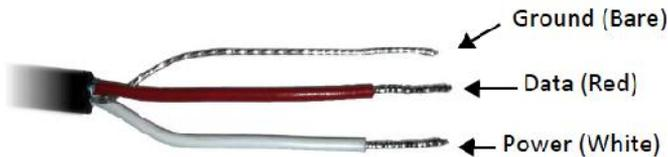
Figure 2: Pigtail Wiring
