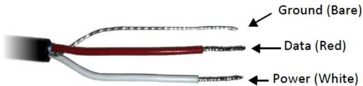
Figure 3: Pigtail End Wiring
