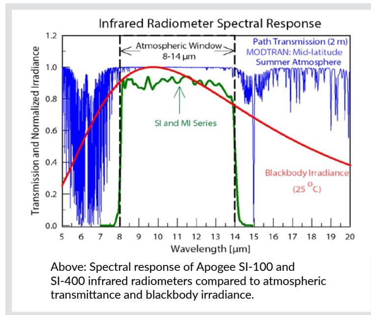
Above: Spectral response of Apogee SI-100 and SI-400 infrared radiometers compared to atmospheric transmittance and blackbody irradiance.
