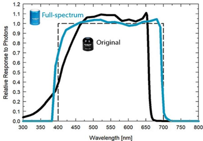
Above: Spectral response of original quantum sensor (black) and full-spectrum quantum sensor (blue) compared to defined response of plants to radiation (dashed).
