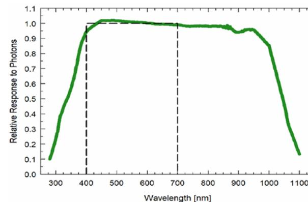
Above: The Quantum Light Pollution sensors have a spectral range of 340 to 1040 nm  $\pm 5$  nm.
