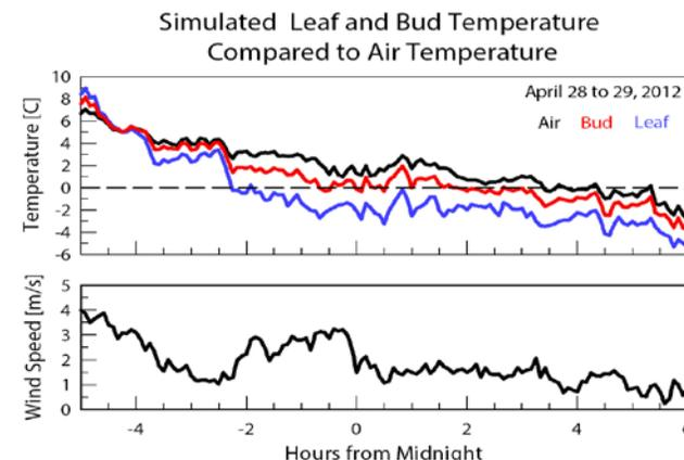
Above: Leaf and bud temperature approximations measured with an Apogee SF-110 compared to air temperature (top panel) and wind speed (bottom panel) on the evening of April 28, 2012. Leaf and bud temperatures were both below air temperature after 8 P.M. and reached freezing 6 (leaf) and 4 (bud) hours before the air temperature.
